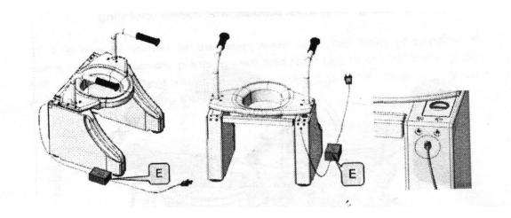
**Warning:** Your Dignity Lifts DL1 requires a GFCI-protected outlet. Be sure to only plug it into an outlet that is GFCI protected. Mixing water and electricity is dangerous, plug your lift in safely.
